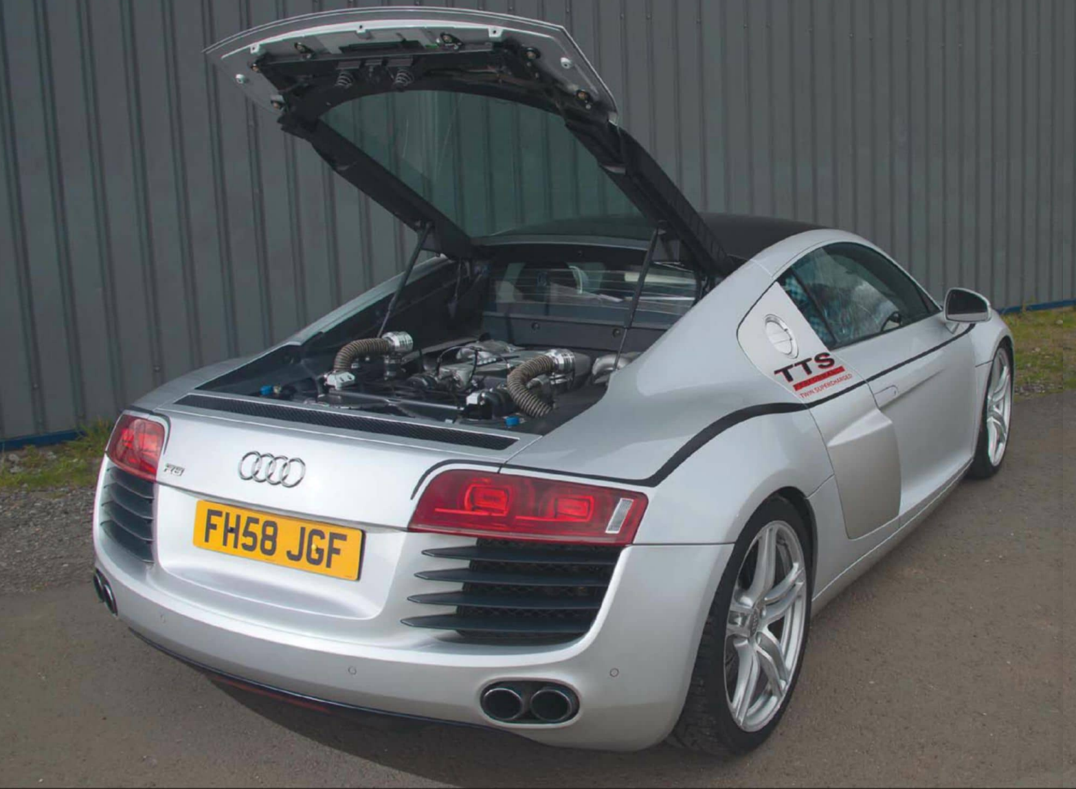
Above The brace of Rotrex C3861 superchargers takes power to a scintillating 750bhp while torque swells to 560lb/ft. To combat the power-sapping heat TTS has developed a highly efficient chargecooler Below Wheels (and brakes) are stock R8s, with 295/30 and 235/35x19 Pirelli P-Zeros
